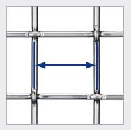
Center-to-Center (CTC) spacing is measured by taking the distance between the center point of two adjacent parallel wires.
