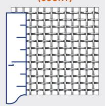
Mesh Count (Count) is the number of openings per linear inch. The example above shows a 7 Mesh.
