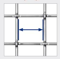
Clear Opening (OPG) of a mesh is measured by taking the distance between two adjacent parallel wires.
