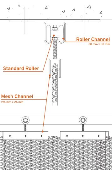
The FOLD FLEXIBLE MESH SYSTEM is comprised of straight profiles at set intervals with rotating hooks that attach to a carriage inside of a heavy-duty zinc galvanized rail. This system allows the flexible mesh to collapse and condense in a uniform arrangement satisfying many aesthetic and functional needs. The rail and straight profiles can be powder coated in a variety of colors, or shipped raw. The Fold Flexible Mesh System is suitable for RIPPLE, NARROWS, and DRIFT.
